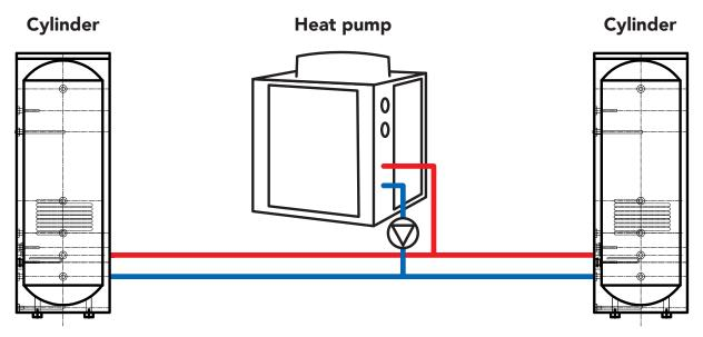
The system is compatible with solar hot water heating options. One heat pump unit can heat up multiple cylinders.
