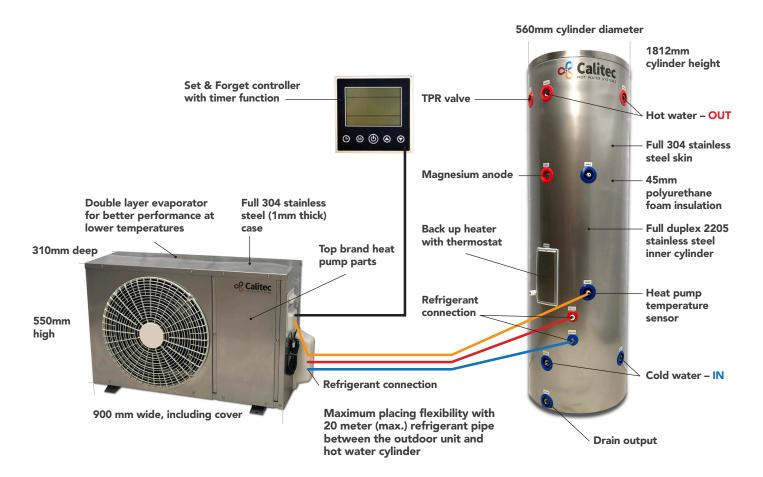
The Calitec Hot Water System is a refrigerant cycling split system with an outdoor unit and a stainless steel hot water cylinder, which fits inside your standard hot water cupboard or you can place it outside.
